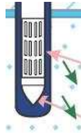
150/200 mm PVC slotted pipes with gravel packing
