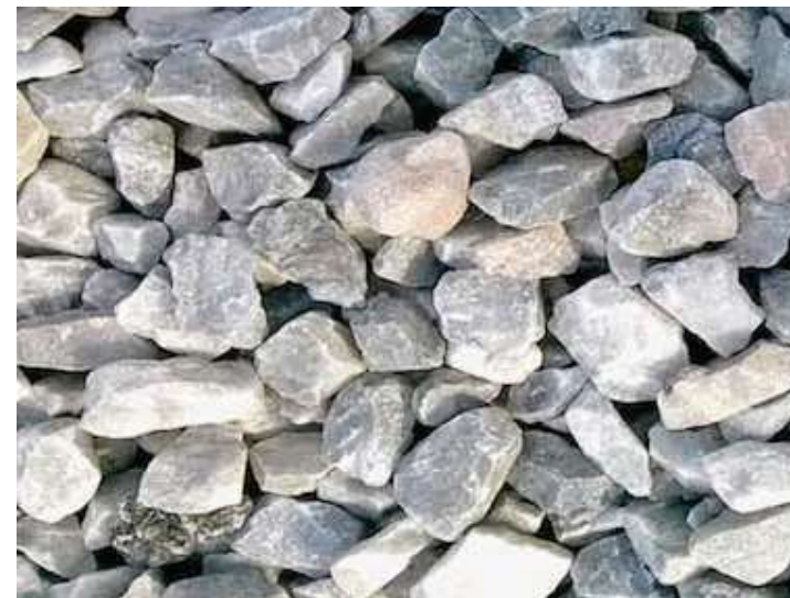
03) Gravels for Adjacent pit filling
